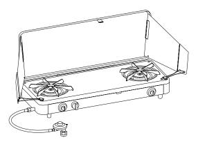
This camp stove is equipped with a hose and regulator to accommodate a disposable propane cylinder. To connect to a larger propane cylinder use Part Number, SHK-4 hose kit.
